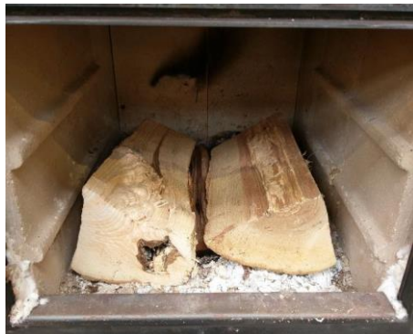
Figure 12 Logs Laid in Firebox
